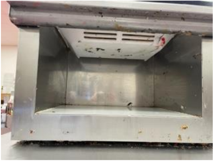
Photo 6 – Dirty interior surfaces to Merry Chef, dirt and debris also trapped underneath equipment
