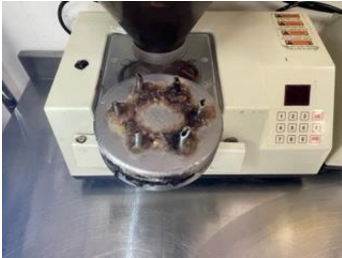
Photo 5 – Dirty needles to doughnut injector
